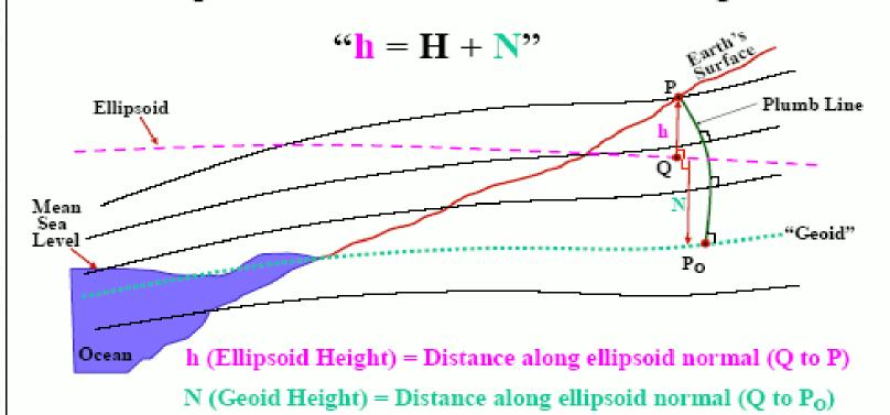
**H** (Orthometric Height) = Distance along plumb line ( $P_0$  to P)
