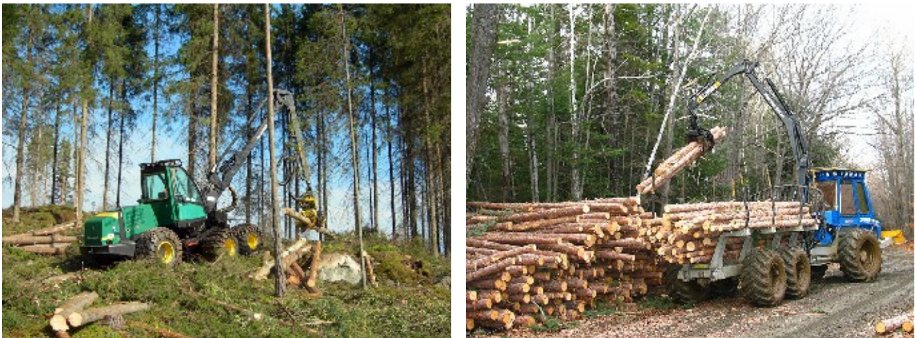
Figure 1. On the left Harvester by Heikki Valve on the right Forwarder by BenFrantzDale, (from
